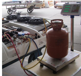
Charging the gaseous refrigerant ,the Refrigerant steel cylinder front stand
